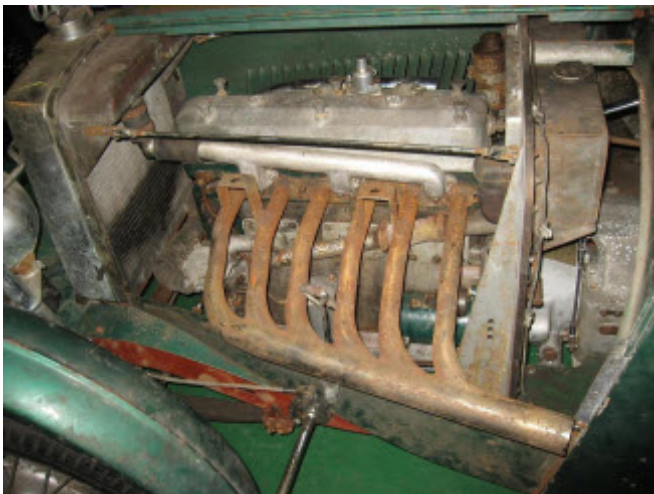
The recent condition of the engine bay, still with the stiffener straps to the exhaust
